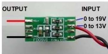
FDDSV1 Voltage Sensor Input Voltage Selection
