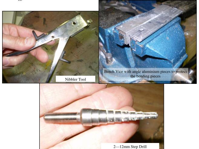
Begin by gluing the templates to the 1.2mm aluminium plate with removable spray glue. The shapes can then be cut out with the nibbler tool. Use a file to smooth up the edges and remove and sharp burrs. The holes should all be drilled at this time. Open up the 30mm holes with the step drill, then use the nibbler and file to finish them off.
