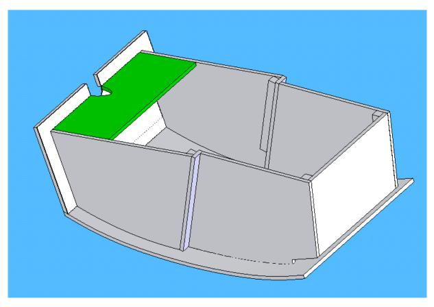
Now glue in the Eye light box bottom. This has a cutout in it to allow the antenna clear access.
