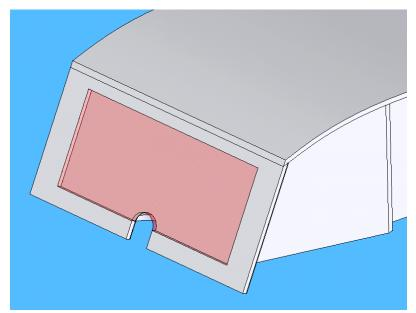
Now cut and file a piece of red Perspex (3mm thickness) (I got mine at Jaycar) to fit snugly into the space in the bezel surround. When you are happy, file out the antenna space as well so it matches the cutout. Leave the protective paper on the Perspex as you will have to paint the head before going further.
