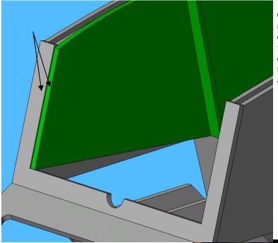
Clamp the assembly so far into the head frame and check it's fit, it should fit snugly and the curve edges should line up with the head frame accurately. If not, file them until they do. With the back clamped tightly, check that the arrowed parts appear to be flush, both left and right sides.
