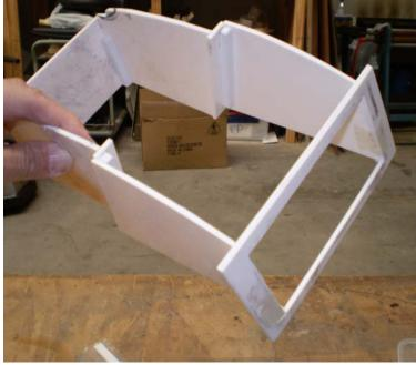
Now glue a 0.5mm sheet to the back of the bezel surround as in the images below and glue the whole thing to the top frame. Make sure you don't get any glue on the 0.5mm styrene. You will be shining 2 eye LEDs through this as a diffuser and glue marks look terrible.
