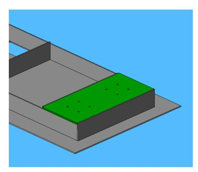
Laminate the 2 Caster Tables together to form a single 6mm thick piece, then glue it into the space provided. From the other side, squirt plenty of glue into the gaps and give it a few hours to set up properly.
