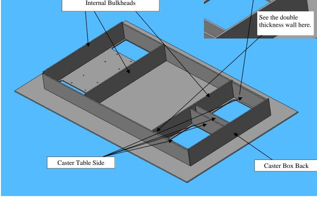
Assemble the pieces as shown, again the lengths and sizes make their location obvious, so no need for a step by step breakdown. Note the 8 holes near the wheels are all 3mm to suit the motor mount assemblies you made earlier.
