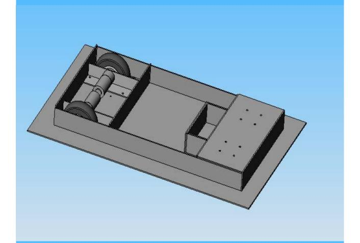
I have 114mm diameter wheels on my K9 so everything is designed around that wheel height. The actual wheels are Du-Bro part 450TL. This is a 4.5inch diameter wheel with a solid foam wheel. These provide a bit of cushioning and grip which is nice.
