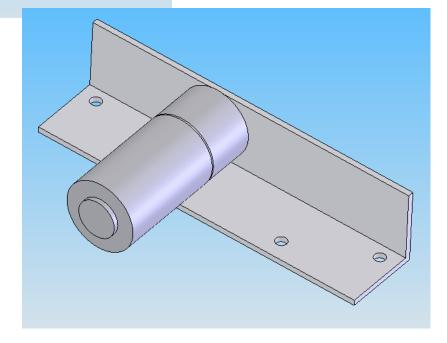
Begin by cutting out the base plate. Chamfer all the edges, it's a bugger of a job but necessary to make things strong.
