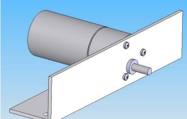
All holes are 3mm except for the large hole which is 12mm. Use a step drill to keep everything accurate.
