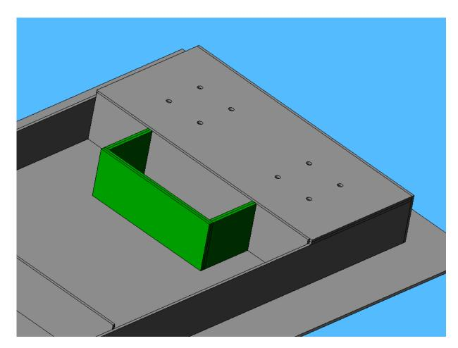
Once everything is setup, you can finally glue the base into the body. After I glued mine in, I cut up some thin strips of 3mm styrene and glued them in against the base and body to add strength. I flooded the area with glue and slid the strips back and forth until they melted into the join.
